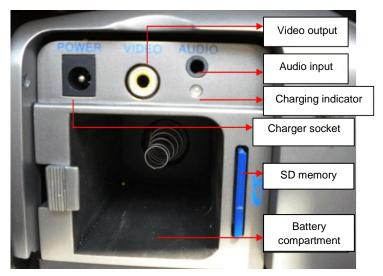
Fig. 15. Arrangement of ports under the cover.
