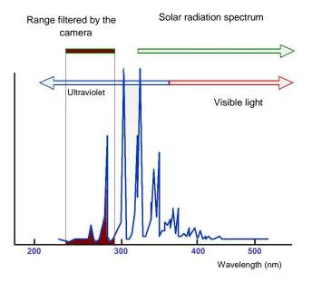
Fig. 2: The spectrum of corona discharge
