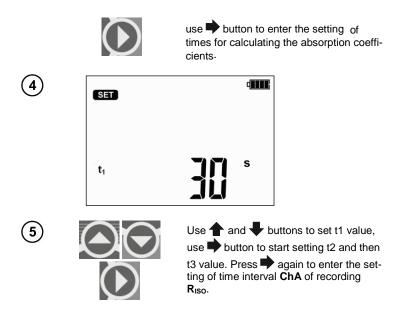
Defining ChA interval will enable the user, using Sonel Reader software, to plot the resistance chart and current chart using the data obtained from the performed measurement (see example below).
