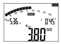
After the measurement is completed or stopped, read the result. The results of all completed measurements will be displayed (even when the measurement was interrupted/stopped e.g. after 60 seconds). When the meter switched into standby mode, the measurement result may be recalled by pressing ENTER.
