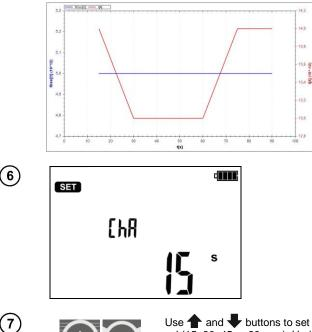
Use **and buttons to set the interval (15, 30, 45 or 60 sec.).** Horizontal lines indicate unavailability of recording characteristics.
