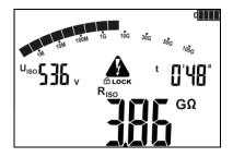
View of the screen during measurement. **LOCK** means that the measurement was started with **ENTER** button or by pressing and holding **START** button for approx. 5 sec.
