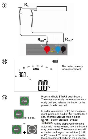
of pre-set t1, t2 or t3 values (measurement without time limit), press again **START** or **ESC** button.
