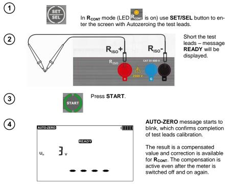
In order to remove the compensation of the leads resistance (return to default calibration), perform the above-mentioned activities with test leads open, instead of test results, the display will show message **oFF** (compensation of test leads is turned off).
