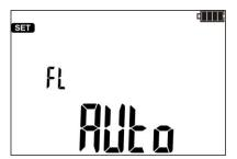
MIC-5001 has an analogue filter which damps variable component of current and allows measurements in an environment with strong electromagnetic interference.
