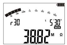
Resistance R<sub>ISO</sub> value, measured in time t=5'30'. Symbol r III indicates the selected time interval, in which the resistance value was recorded.
