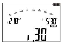
The value of leakage current I<sub>L</sub> measured in time t=5'30'. Symbol 1.30 indicates the selected time interval, in which the leakage current value was recorded.
