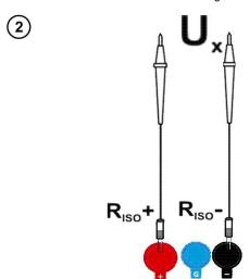
Connect the meter to a voltage source.
