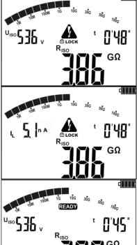
View of the screen during measurement. 1 LOCK means that the measurement was started with ENTER button or by pressing and holding START button for approx. 5 sec.
