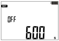
Use buttons and to set Auto-OFF time or to inactivate this function (horizontal lines – Auto-OFF function is inactive). Auto-OFF function is used to turn-off inactive meter after a preselected time (300, 600 or 900 sec.). When the user switches the meter off, it will generate a beep after the set time.
