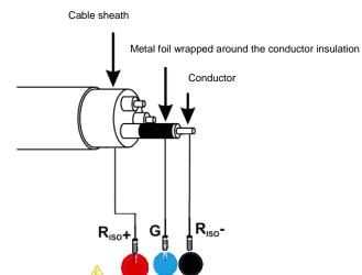
The same shall apply when measuring the resistance between two conductors of the cable, attaching to  ${\bf G}$  terminal other conductors that do not take part in the measurement.
