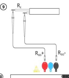
Connect test leads according to the drawing.
