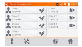
Click, to save data in the USB stick or to copy data from the USB stick to the memory of the meter.
