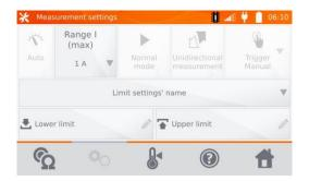
If necessary, select temperature limits from the database (click **Limit settings' name**) or set the required limits for the performed measurement by clicking **Lower limit** and/or **Upper limit**.
