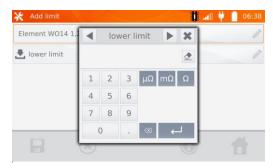
Enter the lower limit. Use button to go to the upper limit setting. You can set only one of the limits.
