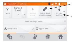
Switching Unidirectional/Bidirectional measurement.
