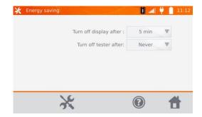
Set the inactivity time for blanking the screen and turning off the meter.
