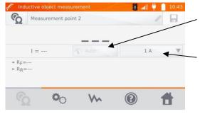
When measuring inductive objects, only Auto mode is available - the measuring current is limited to a value not exceeding the set value,
