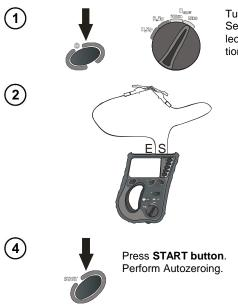
Turn on the meter. Set the rotational function selector at **R**CONT **ZERO** position.
