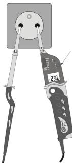
Connect both probes of the tester to a live object
