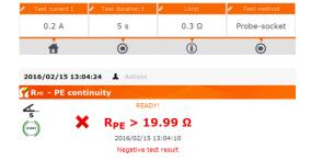
Negative test result: R<sub>PE</sub> > LIMIT
