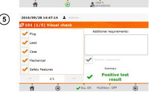
For this example: after initial visual check, select proper fields on the left side of the screen (confirming or not the correctness of the statement). Press
