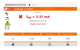
Negative test result: I<sub>PE</sub> > LIMIT
