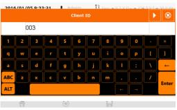
Press , to toggle between next and previous data field without disabling the keyboard. After entering all data confirm the changes by pressing **En-**
