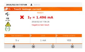
Negative test result: I<sub>T</sub> > LIMIT
