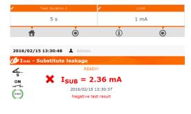
Negative test result: I<sub>SUB</sub> > LIMIT
