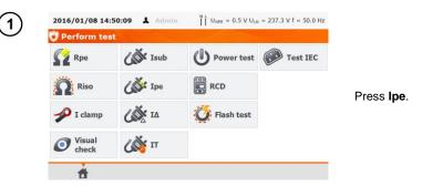
Before starting the measurement, similarly to the measurement of PE resistance test (see 4.2 of this manual), following parameters must be set: **test duration, limit** and:
