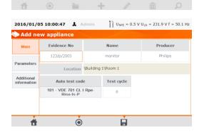
Enter (type) appliance's data in the same way as for the client or object. Filling data marked with orange frame is mandatory. Additional data is available under **Parameters** and **Additional information**.
