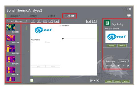
'Report' tab allows to create reports based on taken IR images. Thumbnails of the images that can be put in to the report are shown on the left side of the screen. Upper toolbar contains buttons that allow to add text, note, table and tag or image to the report. On the right side there is information about the selected object in the report. Selected object can also be modified here, for example, line or column in the report's table can be added.
