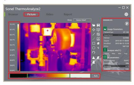
On the left side of the image, temperature scale, where different colors are representing different temperatures, is presented.
