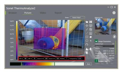
To move the IR image, that sits over visual image, press and hold the left mouse button, and then move the mouse in the desired direction.
