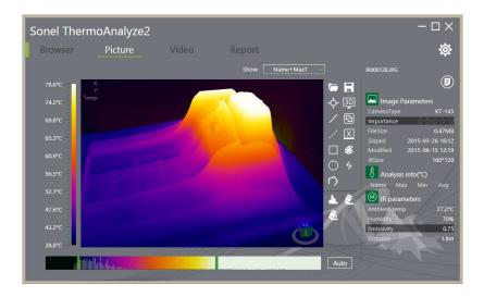
To zoom in or zoom out the 3D view, use the mouse wheel button. Move it up to zoom in the 3D image, and move it down to zoom out.
