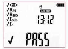
Positive test result for the tested device. The result of each single test of the sequence is positive.
