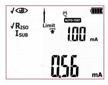
Measurement of R<sub>ISO</sub> insulation resistance has been completed. If the measurement result is negative, further measurements will not be conducted. In case of the positive test result: If the **AUTO-TEST**
