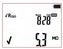
A cell occupied by a single test result. An icon indicating the test type and the main result is displayed on screen.
