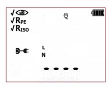
Measurement of insulation resistance has been completed. If the measurement result is negative, further measurements will not be conducted. In case of the positive test result: the tester will automatically run the subsequent tests – polarity check.
