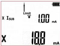
Inorrect result. The value of leakage current is above the set limit. Red LEDs of FAIL indication are on.
