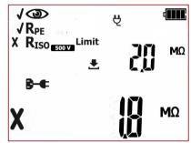
Negative test result for the tested device. One of the subsequent tests has ended with negative result - that result is displayed on screen (screen on the left, as an example, shows failed insulation resistance test). Red LEDs of FAIL indication are on.
