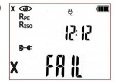
Negative visual inspection result, further measurements will not be conducted. Red LEDs of FAIL indication are on. On the right side of the screen the current time is shown.
