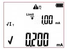
Correct result. The value of leakage current is below the set limit. Green LEDs of PASS indication are on
