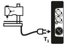
Press START/STOP to commence measurement of protective conductor resistance.
