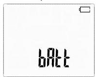
Rechargeable batteries completely discharged.
