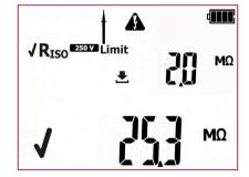
Correct result. The value of insulation resistance is above the set limit. Green LEDs of PASS indication are on.
