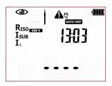
The tester is in autotest mode for Class ш devices. Icons displayed on the left side represent all tests that will be performed. On the right side the current time is shown.
