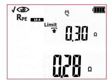
Positive visual inspection result. The tester will automatically run the subsequent tests: R<sub>PE</sub>.
