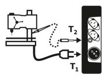
Connection diagram for Class II (III) appliances. The test lead with the probe must be connected to T2 terminal socket. The measurement is made between shorted L and N, and the probe:
