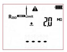
The tester is in insulation resistance measurement mode.
