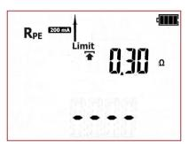
The tester is in PE conductor resistance measurement mode.
