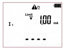
The tester is in touch leakage current measurement mode.
