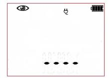
The tester is waiting for the evaluation of the device after completing visual inspection. If the measurement of the L-N circuit resistance is selected, tester will also display the result of R<sub>LN</sub> measurement. If it's not selected, then dashes will be displayed in the main screen area "----".
