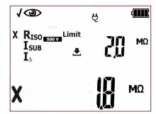
Negative visual inspection result, further measurements will not be conducted. Red LEDs of FAIL indication are on. On the right side of the screen the current time is shown.
