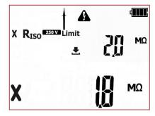
Inorrect result. The value of insulation resistance is below the set limit. Red LEDs of FAIL indication are on
