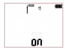
has been measured. M is displayed on the screen. along with the permanent ZERO symbol. After 3 seconds the tester returns measurement mode. The active test lead compensation is indicated by ZERO icon displayed on screen during the tests of R<sub>PF</sub> (200mA, 10A) and CL I autotests. The compensation sistance will be taken into account then displaying test results of Rpf.
