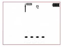
The tester has switched into the test lead compensation mode. ZERO icon is flashing.
