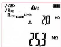
Measurement of PE protective conductor has been completed. If the measurement result is negative, further measurements will not be conducted. In case of the positive test result: the tester will automatically run the subsequent test: R<sub>ISO</sub>.
