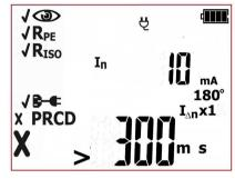
Incorrect result. One or more of the measured parameters are above the permissible threshold. Red LEDs of FAIL indication are on.
