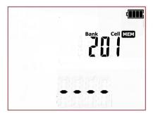
The content of the bank has been deleted, the first cell of the deleted bank is selected.
