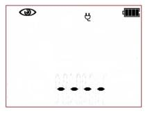
The tester is waiting for the evaluation of the device after completing visual inspection. If the measurement of the L-N circuit resistance is selected, tester will also display the result of R<sub>LN</sub> measurement. If it's not selected, then dashes will be displayed in the main screen area "----".
