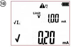
Correct result. The value of leakage current is below the set limit. Green LEDs of PASS indication are on.
