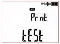
If the code is correct and the connection is properly established, the printer icon will be lit permanently, and the tester will remember the settings and will go to the settings menu (SET) of the tester. If any problem occurs the tester will return to the code input screen (CodE) - verify the correctness of the code and make sure the printer is ready, and then try to connect again.
