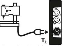
R<sub>L-N</sub> measurement refers to resistive objects, in the case of inductive objects, the result may be subject to additional error
