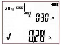
Correct result. The value of PE resistance is below the set limit. Green LEDs of PASS indication are on.
