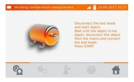
After the desired working time turn off the engine, reconnect the meter to the motor winding and press **START/STOP**.
