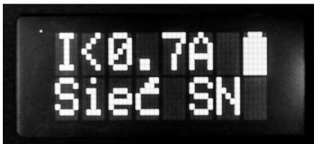
Pic.3 Work in medium voltage mode – alarm limit value and battery level can be seen on the screen.
