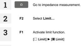
4 LIMIT value ( $\Omega$  Upper 2 /  $\Omega$  Upper 1 / V Lower) is displayed on the measurement screen, i.e.: 04.50m $\Omega$ /03.90m $\Omega$ /10.50V
